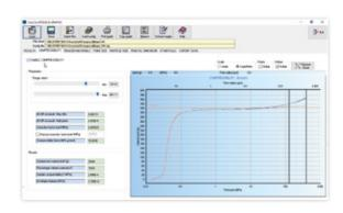
The **PoreInspect software** offers detailed views, here for example the representation of the compression correction
