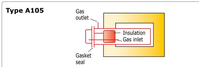
The A105 NiCr alloy (Inconel) retort is sealed by a removable front opening insulated door fitted with a silicone rubber seal. Gas inlet and outlet connections are easily accessible at the front. Oxygen levels down to 30 ppm are achievable. A105 retorts for CWF furnaces are fitted with a 3 mm thermocouple gland through the centre of the door. The retort and furnace must be ordered together as the furnace is modified to allow it to be used with, and without, the retort.
