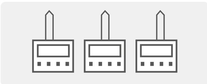
This configuration comprises independent controllers, each with an independent thermocouple in its respective zone. This is the standard method for the TG gradient tube furnaces.
