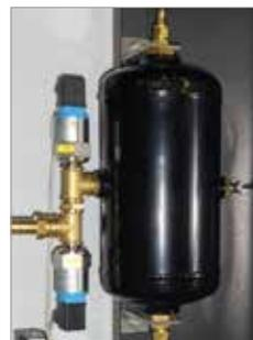
The purging tank is filled with inert nitrogen at a pressure of 8 bar. The purging tank is a required safety option when working with pure hydrogen or other dangerous gases. In case of an emergency this tank provides enough inert gas for purging the whole furnace multiple times to ensure that no dangerous gas remains in the furnace.
