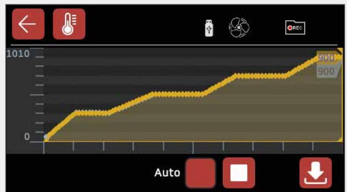
The data logging screen shows a graphical view of the setpoint and actual temperature along with the status of any configured relays. Data is logged to a USB stick in a .csv file format. Data logging can be started manually or automatically when a program is run.
