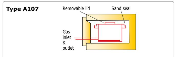
The A107 NiCr alloy (Inconel) retort with a shallow removable lid locates into a sand seal on top of a deep base. Can be used for annealing and pack carburising. Front mounted gas inlet/outlet connections extend through slots in the furnace door.
