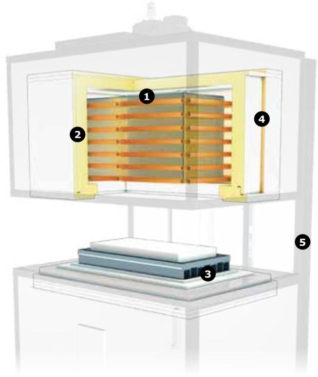
HB-BL 17/430 bottom loader with optional PLC and 19 inch touchscreen control and gas outlet connection to optional catalytical after burner
