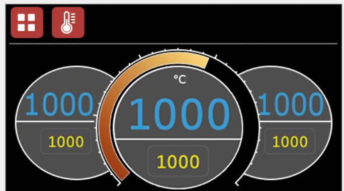
For a 3-zone product the home screen shows the setpoint and actual temperature of each zone. The user can select the end zones to either follow the centre zone temperature or run independently.
