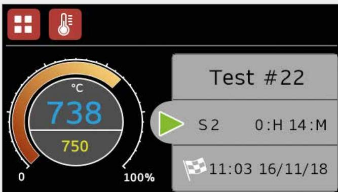
When a program is running the home screen shows a summary of the progress of the program. This includes: the program name; the current program segment and the time remaining in that segment; the end time and date of the program
