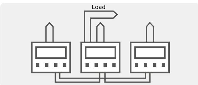
As in single zone furnaces, cascade control allows faster heating of the furnace load and more precise control of the load temperature. A CC-T1, EPC3008P10 or nanodac™ controller is required.
