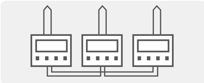
This is the standard method of control for all Carbolite Gero 3-zone furnaces. When the operator adjusts the setpoint of the centre zone controller, the setpoint of both end zones are automatically set to the same value. When a program is run in the centre zone all zones will automatically follow the program. Each controller has one thermocouple positioned with the tip close to the centre of each zone.
