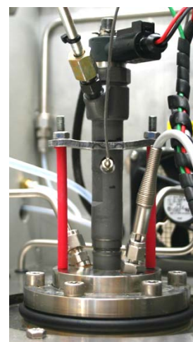
Fig 2: High-pressure fuel Injection system
